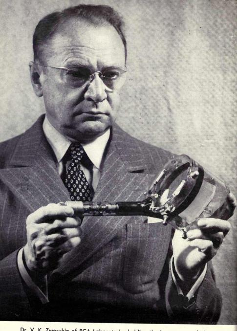
Dr. V. K. Zworykin of RCA Laboratories holding the iconoscope, which he invented as the "eye" of the all-electronic television camera.
